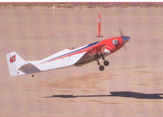
Craig Grunkemeyer is shown with his unlimited racer during a takeoff. Pilots fight a massive P-factor (rolling moment) right after takeoff.
